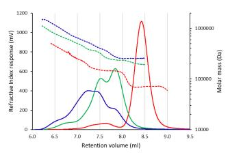
Fig. 1. SEC chromatograms (solid lines) and resultant molecular weight data (dashed lines) for a drug free batch (red), and two active batches (small scale, green, optimised larger scale, blue) of DDC AZD0466, measured in 25 mM aqueous phosphate/citrate buffer at pH 5+glucose 5%w/w.
